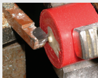
Dentin milled away leaving a protrusion for shear strength testing.
