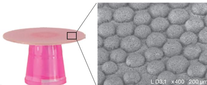
The red Super-Snap X-Treme disks are the first instruments featuring an innovative 3D coating. Between the uniformly distributed semispherical structures made of alumina particles, debris is collected and removed. This reliably prevents the disk from clogging or secondary scratches caused by polishing dust.
